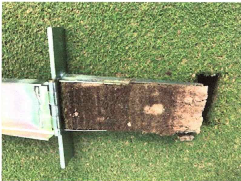
Years of infrequent topdressing and aerification has made the soil retain too much water and soil that is lacking in air space
